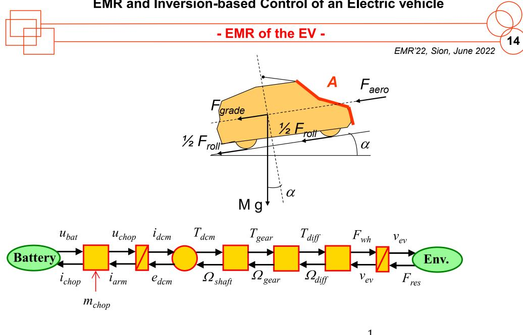
$$F_{res} = k_{roll} Mg \cos \alpha + \frac{1}{2} \rho_{air} A C_x v_{ev}^2 + Mg \sin \alpha$$
