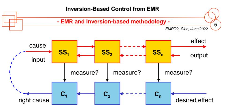
**EMR** = system decomposition in basic energetic subsystems (SS<sub>n</sub>)
