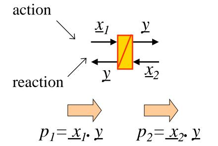
output(s) =  $\int input(s)$  $y \propto \int f(\underline{x}_1, \underline{x}_2) dt$
