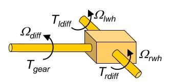
$$T_{Idif} = T_{rdif} = \frac{T_{gear}}{2}$$
